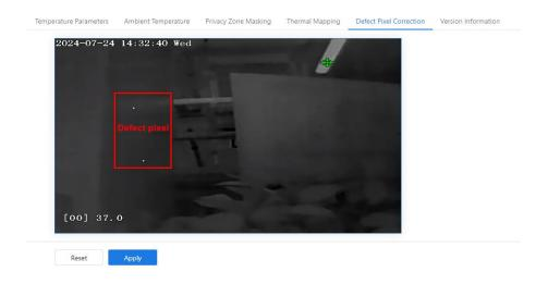
Step 2 Click the white point at image, click **Refresh** to recover the defect pixel, as shown in Figure 4-7.
