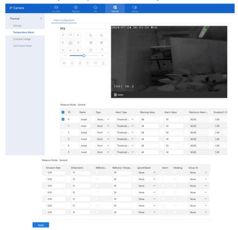
Figure 4-8 Temperature Area and Alarm Configuration
