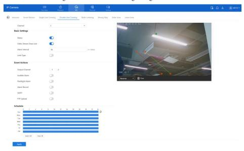
Figure 5-6 Double Line Crossing Setting Interface
